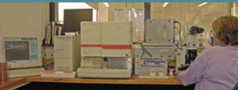
At centre is the IRIS iQ200Elite automated analyser with computer screen to the left. A medical laboratory scientist is demonstrating the manual method of urine analysis that was used in the past at Canterbury Health Laboratories.
